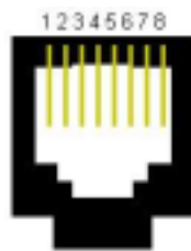
Figure 2-21 RJ-48 Port Pin Order
